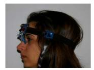
The eye tracker only looks at the eyes and does not record a video image of any part of your face. The total length of the testing is about 30 minutes and detailed instructions about the task will be given to you before the beginning of the experiment. At the end of the experiment you will be asked a few simple questions about your symptoms and asked to make some simple movements in order to assess your condition clinically.
